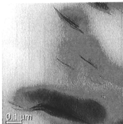
Figure 5. TEM image of cryofracture surface for PP composite with 5 wt% Cloisite Na + and 1% poly(ODA-grad-MAH) (23) additive (reproduced with permission from reference (32). Copyright 2006 Wiley-VCH).
